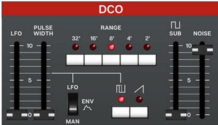
DCO-106 accurately models the unique master clock and divider architecture used in the original Juno synth oscillators, as well as the quirks of the waveform shapes.
