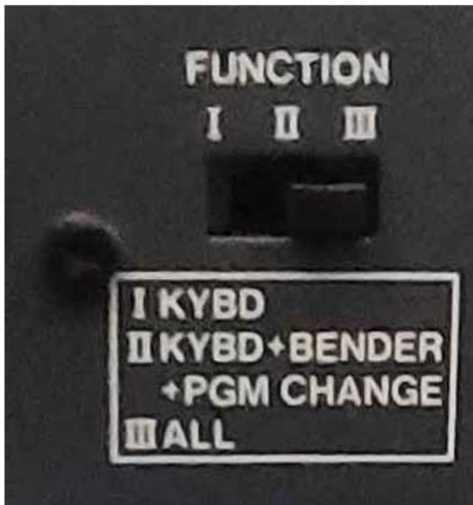
The *Function* switch on the Juno-106's back panel needs to be set to the *III* position for all this magic to work. Note that because it uses MIDI System Exclusive data, MIDI channel settings won't affect its operation (MIDI SysEx is not channelized and will not have unintended effects on other instruments or plug-ins.)
