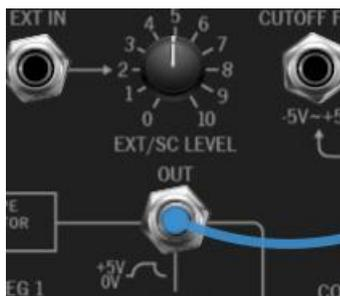
Now let's examine an output. Envelope Generator 1 is normally routed to VCO 1 and VCO 2 pitch (with its mod amount controlled by the *VCO 1 EG1/Patch Panel* and *VCO 2 EG1/Patch Panel* attenuators in the *Frequency Modulation* section beneath the Mixer). If a cable is plugged into the Envelope Generator 1 *Out* jack, its control signal can be routed to any other CV input. **Unlike a CV input jack, CV outs are multed, so plugging a cable in has no effect EG1's hard-wired internal connections.**
