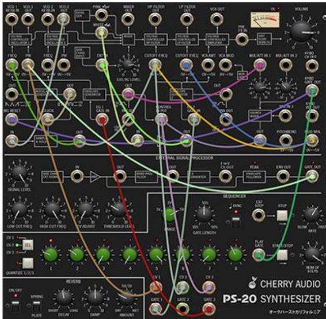
The Patch Panel may appear to be a terrifying mess of jacks, but we promise, it isn't too hard to understand, and unlike a fully modular synth, PS-20's semi-normalled connection scheme makes it easy to use only patching that you need, while leaving the rest of the instrument operating like a standard non-modular synth.
