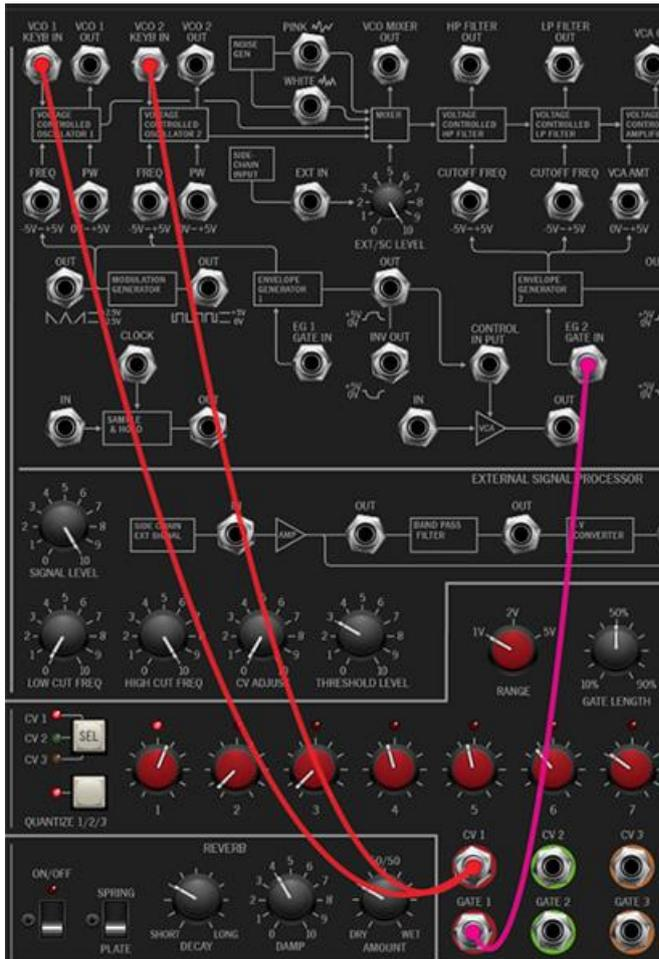
The patch shown above is good starting point. It uses the first sequencer channel with *CV 1* patched to *VCO 1* and *VCO 2 Keyb In* jacks to control pitch, and the *Gate 1* jack patched to the *EG 2 Gate In* jack. Once you have it patched, click the *Start/Stop* button, and turn the knobs to hear varying pitches. You may want to experiment with pitch range and octaves using the *VCO Scale* knobs and sequencer *Range* knob, respectively.
