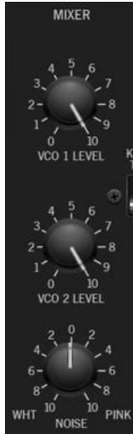
**VCO 1 / VCO 2 Level-** The *VCO 1 Level* and *VCO 2 Level* knobs adjust the volumes of each oscillator.
