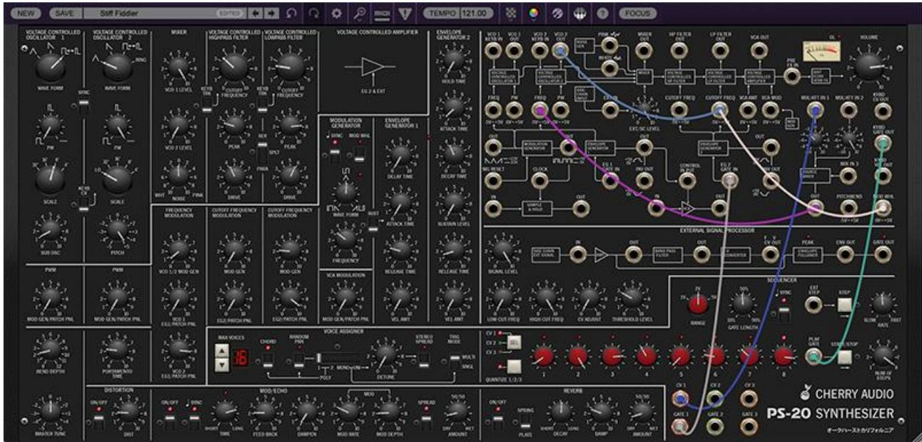
At the most basic level, the original MS-20 has a relatively simple voice architecture: it's a monophonic (one-note-at-a-time) analog synthesizer with two oscillators mixed into highpass and lowpass filters in series (one after the other), then to a VCA, which is controlled by an envelope generator. There's also an additional simple envelope generator that normally modulates the pitch of both oscillators, and an LFO that controls both oscillator pitches and/or filter cutoff frequencies.
