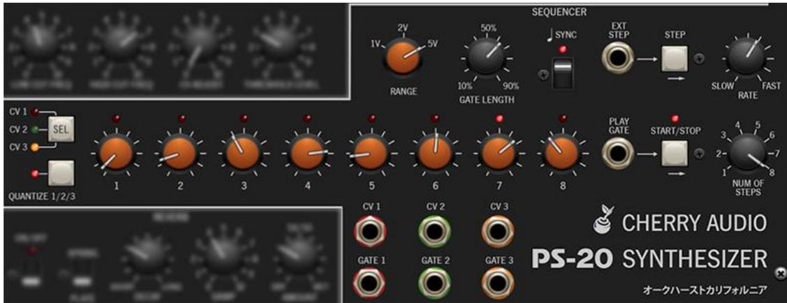
**Channel Sel button and LED's-** Clicking the *Sel* button cycles through each of the three channels. Not only will the LED next to the button glow to indicate the current channel, the CV and *Range* knobs also change colors.
