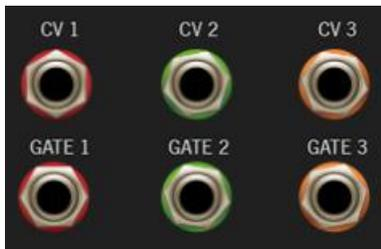
**CV 1, CV2, CV3 out jacks**- The output jacks for each channel of sequencer knob CV's.
