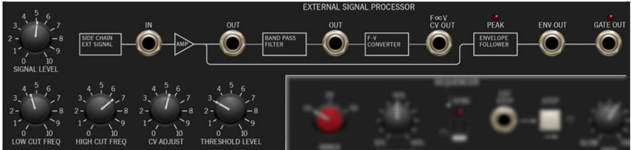
The External Signal Processor analyzes incoming audio and generates matching voltages for controlling oscillator pitch and envelope amplitude, letting you "play" Voltage Modular by singing, playing guitar, or any other monophonic signal source. PS-20's frequency converter has a much wider range than the original for increased functionality, while still retaining its inherent quirkiness.
